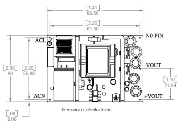
30W Ultraminiature Open Frame Switching Power Supplies
